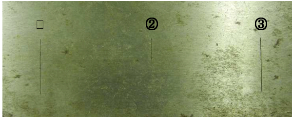
Fig. 9 Target piece with three defects.
