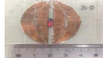
(b) Planar semicircular exciting \infty coil
